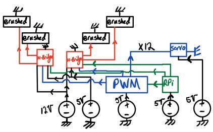
Fig B1. Full Motor Control Circuit Schematic [27]
