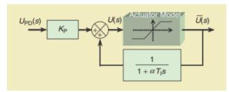
Fig 9. Common PID Controller Schematic [21]
