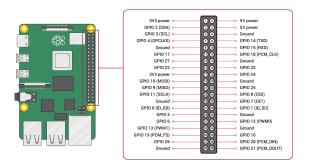
Fig 7. Rpi 4 Pin Layout [19]
