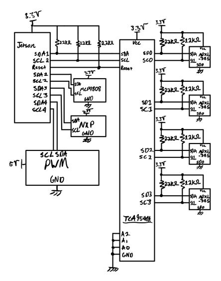
Fig B2. I2C Circuit Schematic [27]
